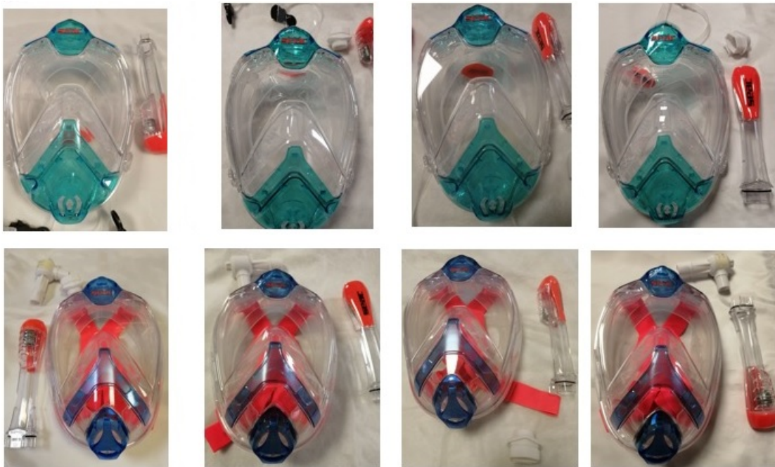
Figure 8 Top the mask SEAC Libera, bottom the mask SEAC Unica. On the left the masks before the cycles, moving to the right the masks after each cycle.
