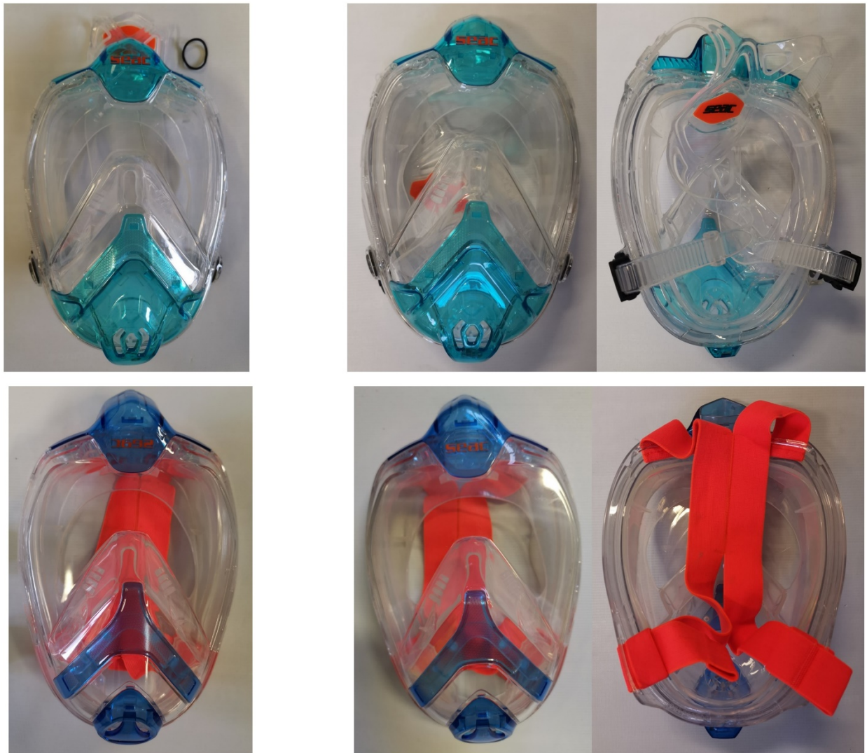
Figure 7 Top the mask SEAC Libera, bottom the mask SEAC Unica. On the left the masks before the cycles, on the right the masks front and back sides after the cycles.
