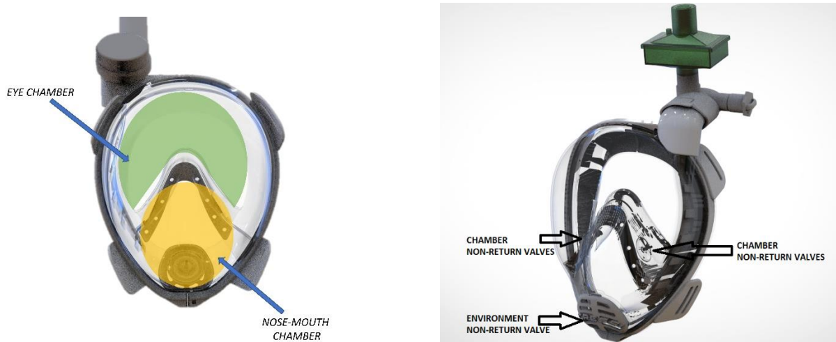
Figure 2 Left: hermetic spaces. Right: non-return valves.
